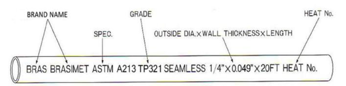
The stencil mark is available for each pipe and tubing of outside diameter exceeding 7mm.
