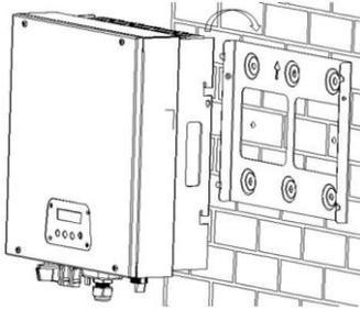
4. Check both sides of the inverter to ensure that it is securely in place.
