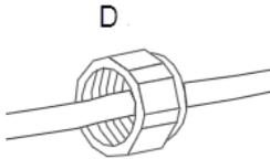
3. Guide the threaded sleeve (B) with the sealing ring over the AC cable.
