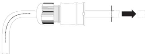
6. Shorten the line conductor L and neutral conductor N by 4 to 5 mm.
