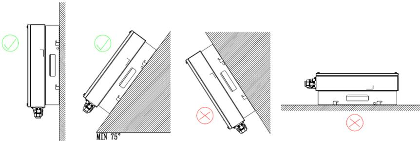
1. Mount the inverter vertically or tilted backward by a maximum of 15°.
