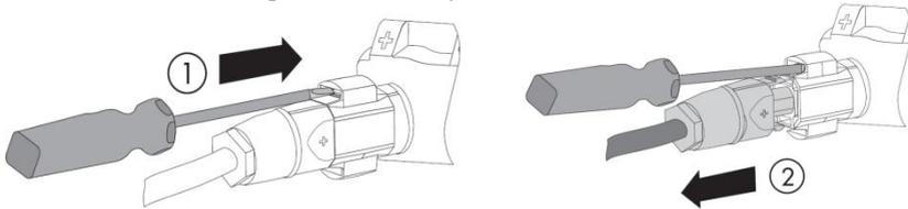
5. Release and disconnect the AC connector. To do so, insert a flat-blade screwdriver (blade width: 3.5 mm) onto the spring clamp and pull the AC coupling plug out of the AC connection receptacle on the inverter. Do not pull on the AC cable.
