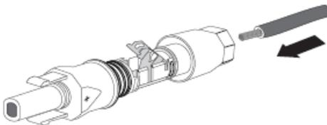
3. Press the clamping bracket down until it audibly snaps into place.
