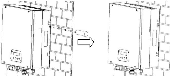
If a second protective conductor is required in your country, ground the inverter and secure it so that it cannot be lifted off the wall bracket (see section 5.4.3 “Second protective grounding connection”).
