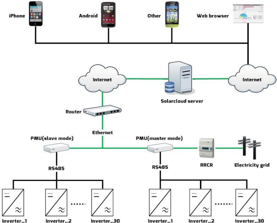
The PMU connects to the inverter via the RJ45 interface, and it connects to the router via Ethernet.
