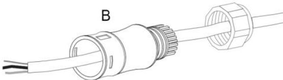
4. Bend the AC cable. The bending radius must be at least four times the cable diameter.
