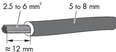
2. Route the stripped cable all the way into the DC connector. Ensure that the stripped cable and the DC connector have the same polarity.
