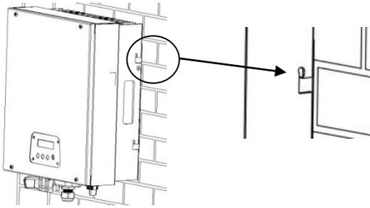
5. Push in the inverter as far as possible and attach it to both sides of the wall bracket using the M5 screws and washers.
