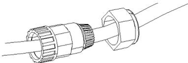
3. Strip the cable's outer sheath (72mm) and the conductors' insulation (9mm).
