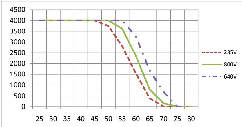
Power reduction with increased ambient temperature (TLC5000)
