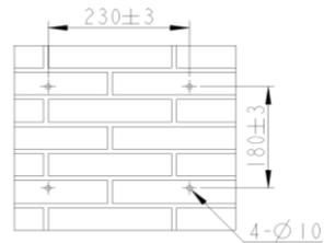
2. After cleaning the dust and other objects from the holes, place 4 wall anchors into the holes, then attach the wall bracket to the wall using the hexagon head screw delivered with the inverter.
