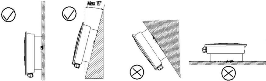
1. Mount the inverter vertically or tilted backward by max. 15°.
