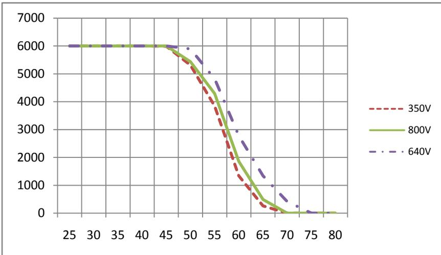
Power reduction with increased ambient temperature (TLC8000)
