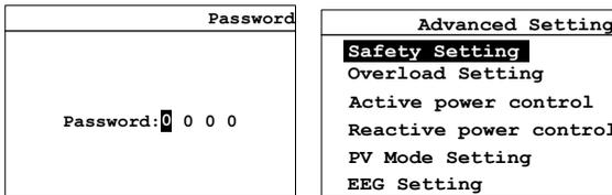
At the "safety" page, use the "▲" or "▼" button to adjust the selected parameter and confirm with the "↵" button, then adjust the next parameters in turn. Parameter adjustment will be finished after the "↵" button has been pressed. Press the "ESC" button to cancel.
