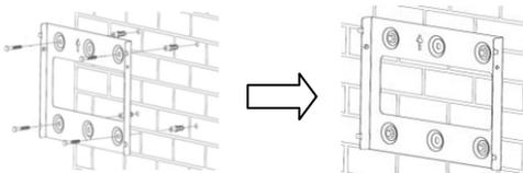
3. Hold the inverter using the handles at the corners, attach the inverter onto the wall bracket tilted slightly downwards.
