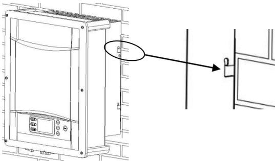
5. Attach the outer fins of heat sink to both sides of the wall bracket using M5 screws. (screw driver type: T25, torque: 2.5Nm).
