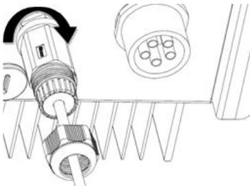
5. Push the seal into the threaded sleeves, screw the swivel nut to the threaded sleeve tight by hand.
