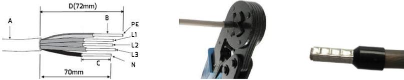
5. Insert the crimped conductors L1, L2, L3, N and PE into the corresponding terminals and tighten the screw with torque 2.0Nm using an Allen key (AF 2.5).
