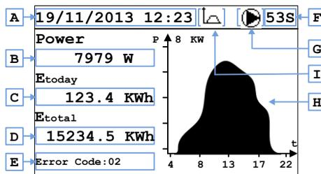
The LCD will switch to standby mode and jump to the home page automatically, and the backlight will turn off when there is no button operation in 30 seconds.
