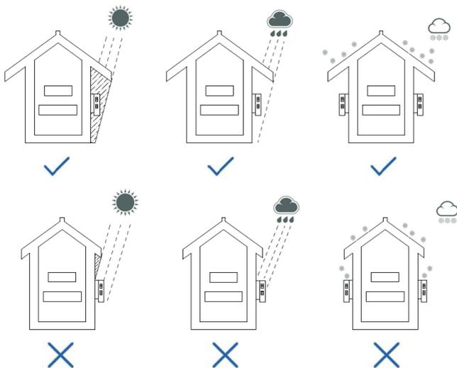
8. The mounting method, location and surface must be suitable for the inverter's weight and dimensions.
