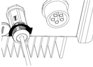
Disassemble the RJ45 plug:
