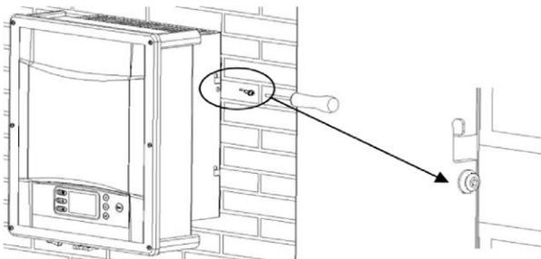
If a second protective conductor is required locally, ground the inverter and secure it so that it cannot be lifted off the wall bracket (see section 5.4.3 “Second protective grounding connection”).
