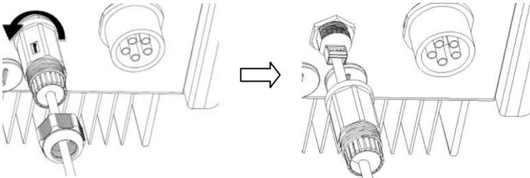
3. Remove the network cable and then screw the cap nut to the RJ45 keystone socket by hand.
