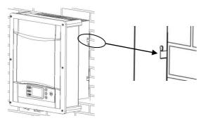
5. Attach the outer fins of heat sink to both sides of the wall bracket using M5 screws. (screw driver type: T25, torque: 2.5Nm).
