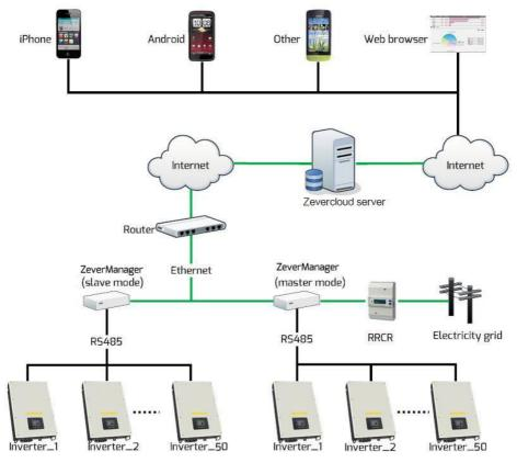
ZeverManager connects to the inverter via the RJ45 interface, and it connects to the router via Ethernet. Then you will be able to connect the inverter to the remote monitoring platform "ZeverCloud". You can monitor the operating status or power
