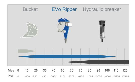
EVo Ripper is exceptionally suitable for soft to medium hard rock like limestone, sandstone and basalt, as well as reinforced concrete.
