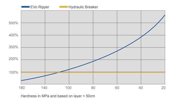
The EVo Ripper combines the working principles of impact force of a hydraulic breaker with vibration and ripping power of a conventional ripper. Due to this combination of both breaking, vibration and ripping, it can produce up to five-times higher excavation rates compared to conventional hydraulic rock breakers.
