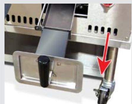
Pull-out drawer to dispose used wood chip
