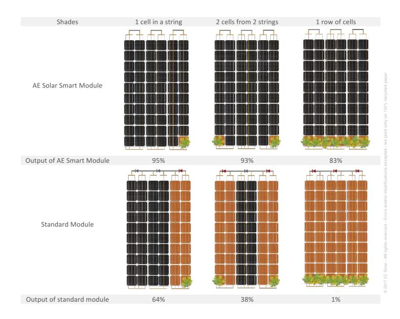
When multiple cells are in shade, a hot-spot free module can generate 80% more power, compared to a standard module.
