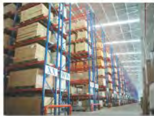
Bangkok Franchise Warehouse Selective Racking
