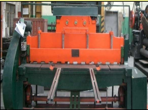
Bending Machine Thickness: 2mm Length: 2440mm Tons: 100 Tons
