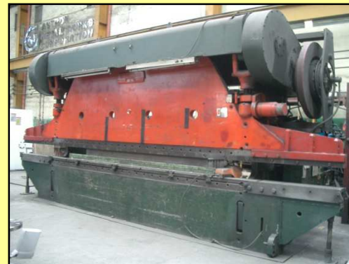
Press Brake Cincinnati Thickness: 3mm Length: 3650mm Tons: 220 Tons
