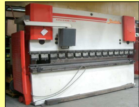
Bending Machine Thickness: 20mm Length 3100mm Tons: 160 Tons
