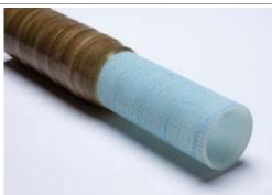
The PVDF HV-Liner from AGRU is an economical alternative to traditional fabric backed pipe. The surface-treated PVDF pipe has a three-dimensional surface structure that provides for optimal bonding with the GRP pipe. The piping systems are available in PVDF, PVDF-FLEX and PVDF-el. The pipes can be produced in diameters from 20 – 355 mm.
